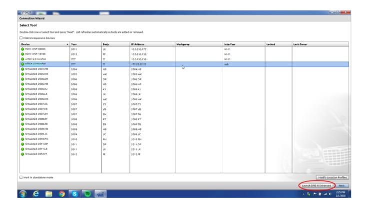
4. Click the "Launch DRB III Enhanced" button and accept the EULA that is presented. A warning will be presented indicating that Enhanced DRB III Emulator is not installed. Press "OK" to start the installation process.
